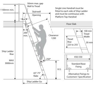
Min dimension between handrails 540mm
